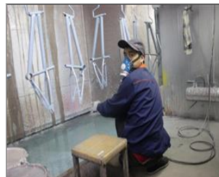
Photo of non-conformity NC-No goggles was used by one spray painting worker.JPG
