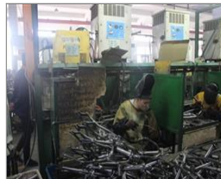
Photo of non-conformity NC-No anti dust mask was used by one welding worker.JPG
